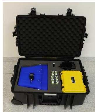
Fig. 2 3D-Scanner prototype in travelling case
