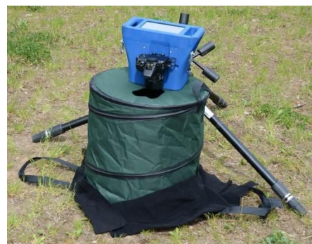
Fig. 4 Scanning with the 3D-scanner using tripod and shadow box under bright outdoor conditions
