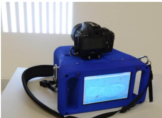
Fig. 1 Complete prototype 3D-scanner
