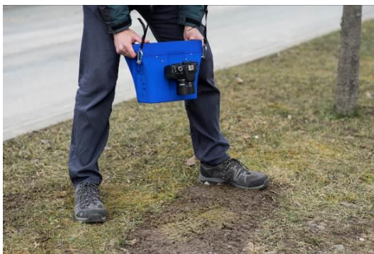
Fig. 3 Handheld scanning with the 3D-scanner
