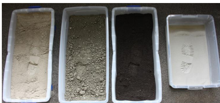
Fig. 11 Boxes with different ground materials, from left to right: sand, clay, soil & mortar
